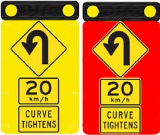
Figure 4.36: Compound curve warning sign with flashing lights
