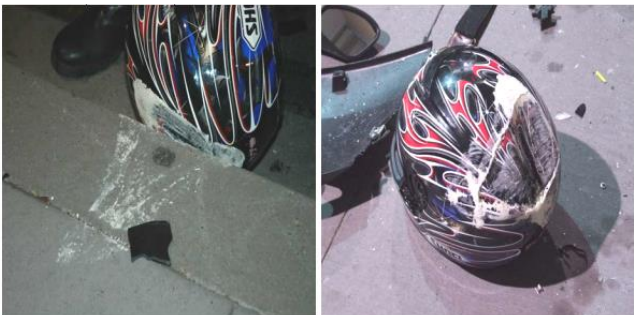
Figure 4.116: Concrete barrier kerb impact on helmet
