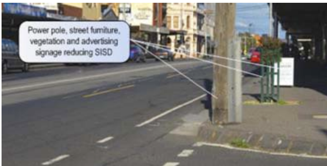
Figure 4.78: Urban – restricted safe intersection sight distance
