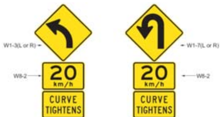
Figure 4.35: Compound curve warning signage
