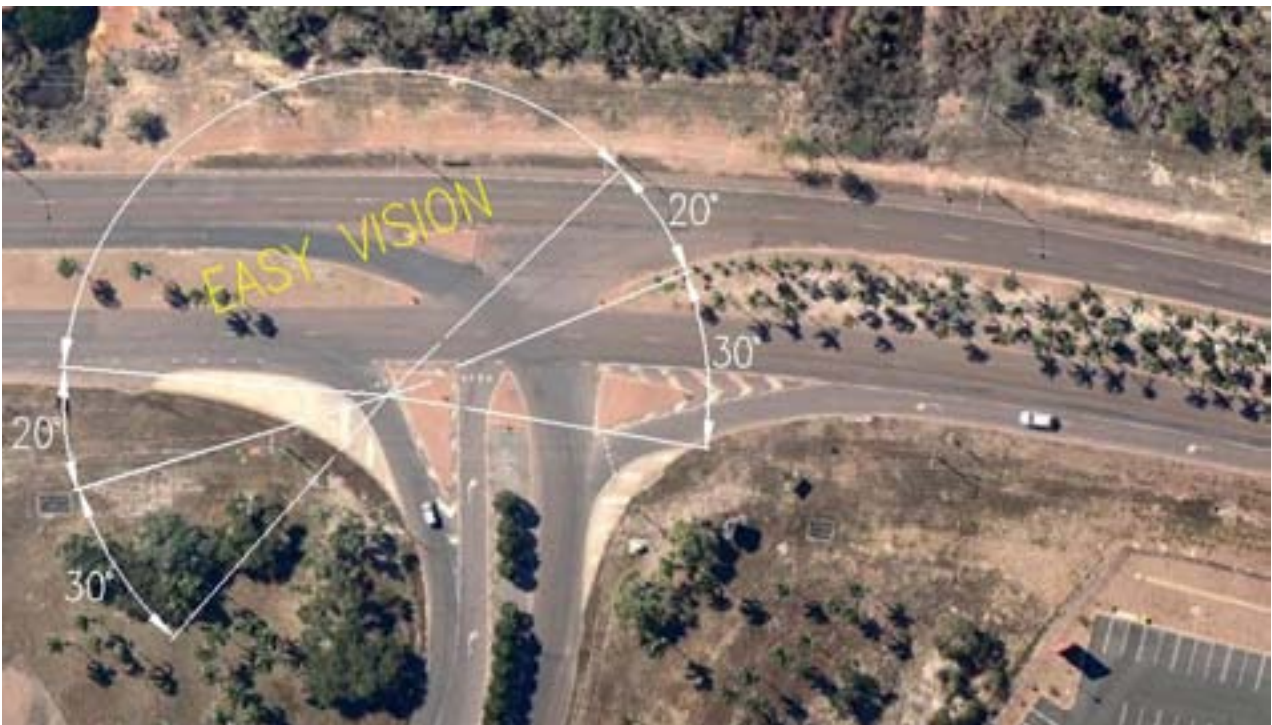
Figure 4.84: Poor visibility angles to through road
