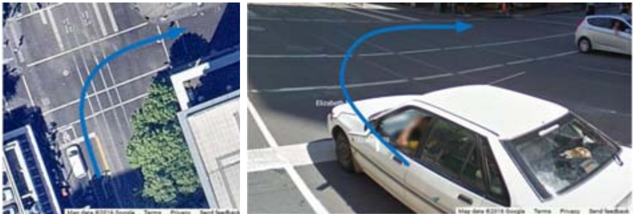
Figure 4.75: Tram crossing, tracks on the turning path
